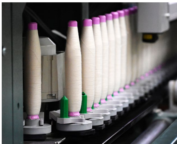
Fig. 3: 12% faster cop transport with SERVODisc
