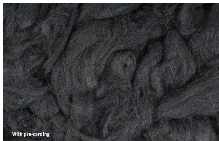
Fig. 1: The pre-carded material contains no yarn pieces, which improves the spinnability of the recycled material.
