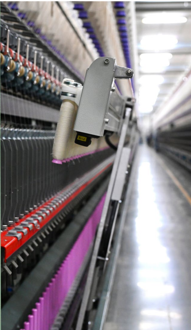
Fig. 1: The latest G 38 doffs in just 90 seconds, which leads to a production gain.
